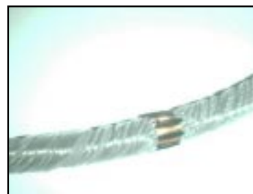
Figure 3 - Close-up view of the pressure sensing system fitted over the shaft of the colonoscope
