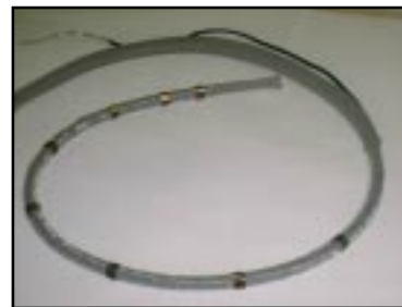
Figure 2 - Overall view of the pressure sensing system fitted over the shaft of the colonoscope
